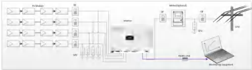
Fig 5.1 Connection diagram for PV grid-connected system
