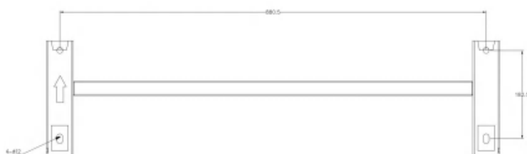
Fig 4.6 dimension drawing of installation hanging plate
