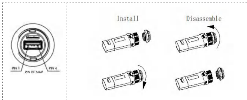
Figure 6.5 Communication interface and installation and disassembly diagram
