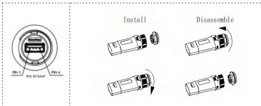
Figure 6.2 Communication interface and installation and disassembly diagram
